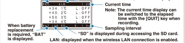
Note: The current time display can be switched to the elapsed time with the [QUIT] key when recording.
