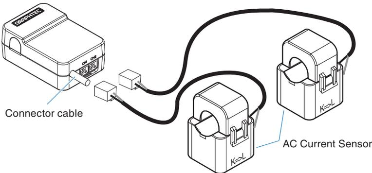
**WARNING** The connector is exclusively to be used to connect the AC Current Sensor. Do not connect it to voltages, other electrical currents, etc. It will damage the module.
