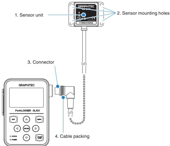
1. Sensor unit ..... The 3-axis acceleration and temperature sensor are built in this module.
