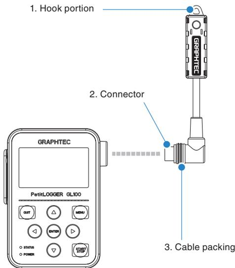
1. Hook portion ..... Used to mount to a wall.
