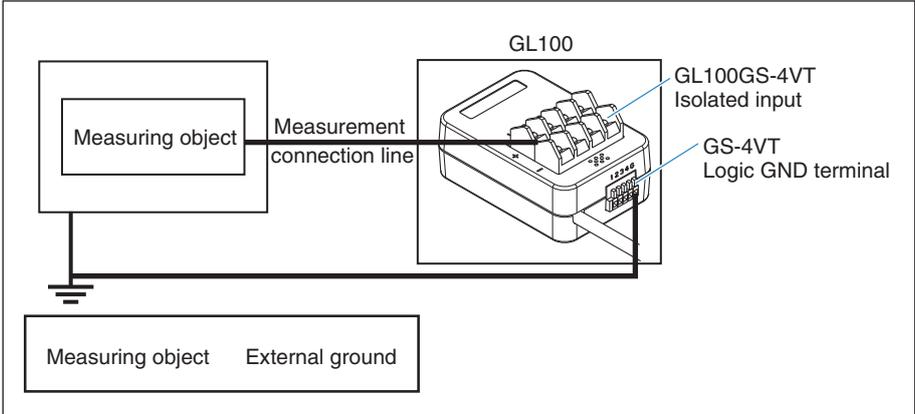
The diagram illustrates the connection setup for the GL100 module. A box labeled 'Measuring object' is connected to the 'GL100' module via a 'Measurement connection line'. The 'GL100' module features a 'GL100GS-4VT Isolated input' and a 'GS-4VT Logic GND terminal'. The 'Measuring object' is also connected to an 'External ground' symbol, which is represented by a vertical line with three horizontal bars at the bottom.
