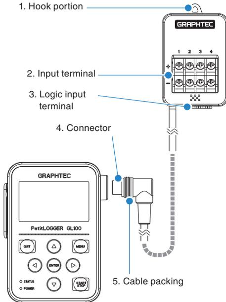
1. Hook portion ..... Used to mount to a wall.
