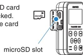
When ejecting the microSD card, push it in gently, then remove the card.
