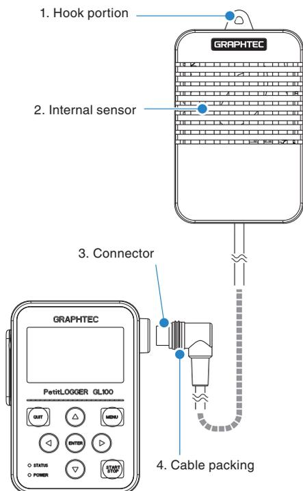
1. Hook portion ..... Used to mount to a wall.
