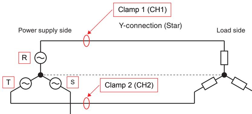
Note: If the current flows in the neutral conductor in the Y-connection, the measurement error occurs because the sum of the three phase currents is not zero.
