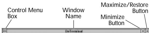
The DTWin title bar is the strip across the top of the application window. It contains the window's name, the Control menu box, and two sizing buttons.
