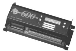
The Datataker 600 is a microprocessor based battery powered data logger which measures inputs from most sensor types. Data manipulation includes statistical functions, calculations and sensor calibration. Data is stored in battery backed RAM and removable memory cards. Alarms can be set for all channels. The Datataker 600 has an integral display and keypad. Suitable for scientific, industrial and public utility applications.
